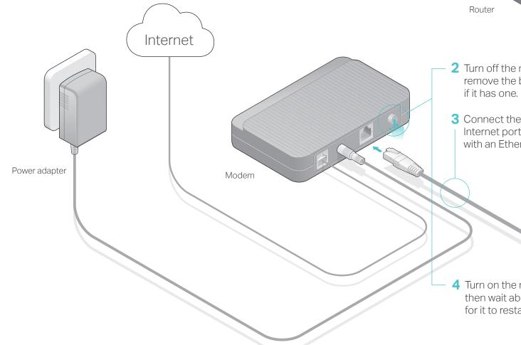
2 Turn off the modem, and remove the backup battery
